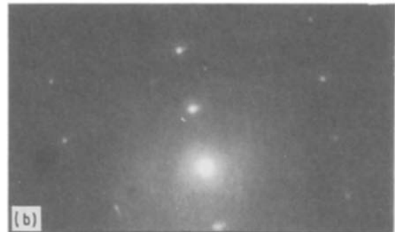
Figure 8 Transmission electron micrographs of alloy 3: (a) morphology of second-phase precipitates in the grain centres ( \times 50\,000 ) and (b) their selected-area diffraction pattern.
